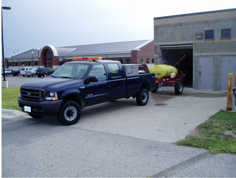
FIGURE 6.1. Pest Management Vehicle with 300-Gallon Boom-Sprayer
